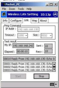
The "LINK" tab is similar to the Ping Command. It allows you to monitor transmission quality between two stations. Enter the IP address of another station, set the timeout and packet size to see if the communication was sent successfully.
